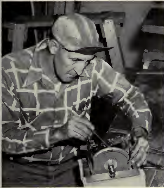
SIMILAR TO A THERMOSTAT, the automatic gate tender raises and lowers the gates according to the amount indicated on the turnout settings. Here Glenn C. Beach puts together the float pulley-cam unit at the Bureau shop. This unit is operated by a float.
